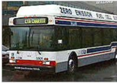
P3 BUS - 205 Kw. CHICAGO & VANCOUVER
